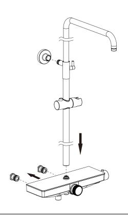
Insert the Tighten Bracket tube of the adjustable base into the fixing base . Adjust the distance between the slide bar and the finished wall and tighten the nut in the fixing base.
