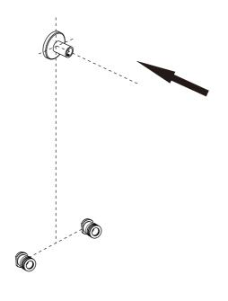
Connect the shelving tap to the wall joint and lock it withscrews from the bottom.
