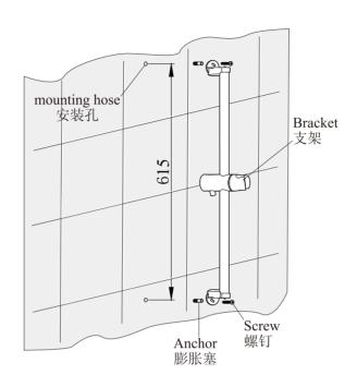
As is showen in the picture, screw the self-tapping screws into the anchors though the sleeve. Tighten them by screwdriver.
