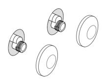
Insert washer seals into supply nuts of the faucet. Thread the faucet supply nuts onto the connectors and tighten.
