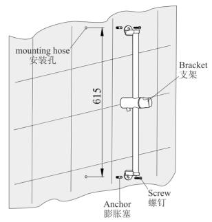
As is showen in the picture, screw the self-tapping screws into the anchors though the sleeve. Tighten them by screwdriver.
