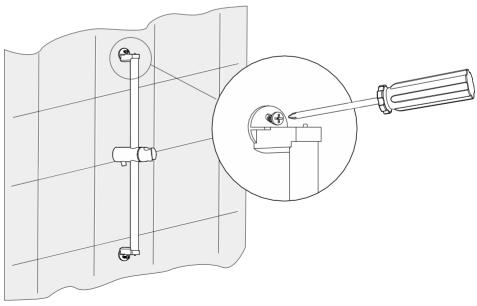
As is showen in the picture, Slide the bracket and onto the sleeve and insert the locking pin into the hole of the bracket and sleeve.
